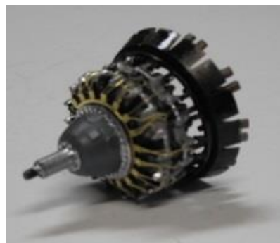
One of the two Pratt & Whitney R2800-65 Double Wasp engines
