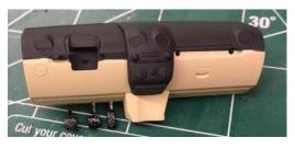
Once the interior Buff paint was dry, Bill flocked the interior tub with tan, and used a Flory wash (from Flory Models) in the seats. He then masked the inside of the windows using the kit supplied masks. The masks are to allow for painting the black border around the windows. Since the windows are installed from the inside, they must be masked prior to any painting.
