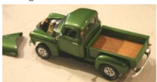
& whistles under the hood. He made his home exhaust system and finished it off with aluminum tips. The body was airbrushed a Dupli-color spray can green he decanted. The wooden bed was a wood used for dollhouses.
